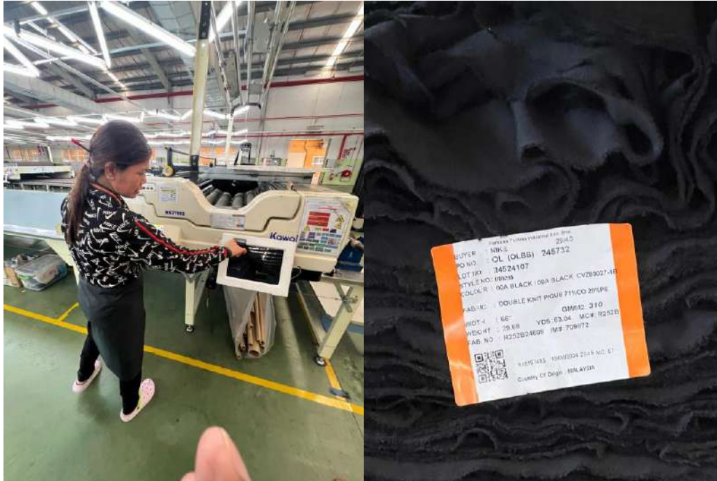
Example 1: QR code at cutting table for fabric identification
